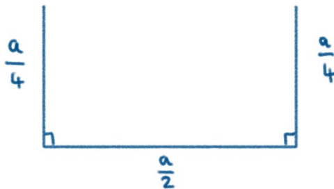
Figure 3 - Diagram to show the ratio of the sides in an optimum rectangular gutter
